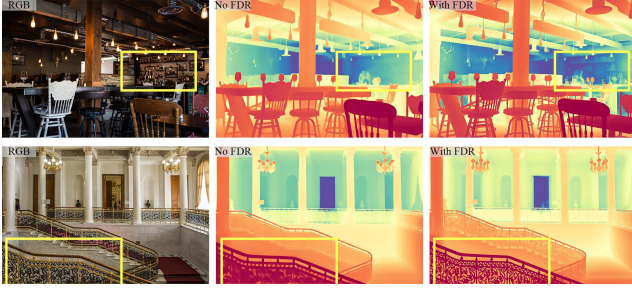
Figure 3: Illustration of our specially designed frequency-domain loss function, which effectively enhances high-frequency edge details in the predicted depth maps.
